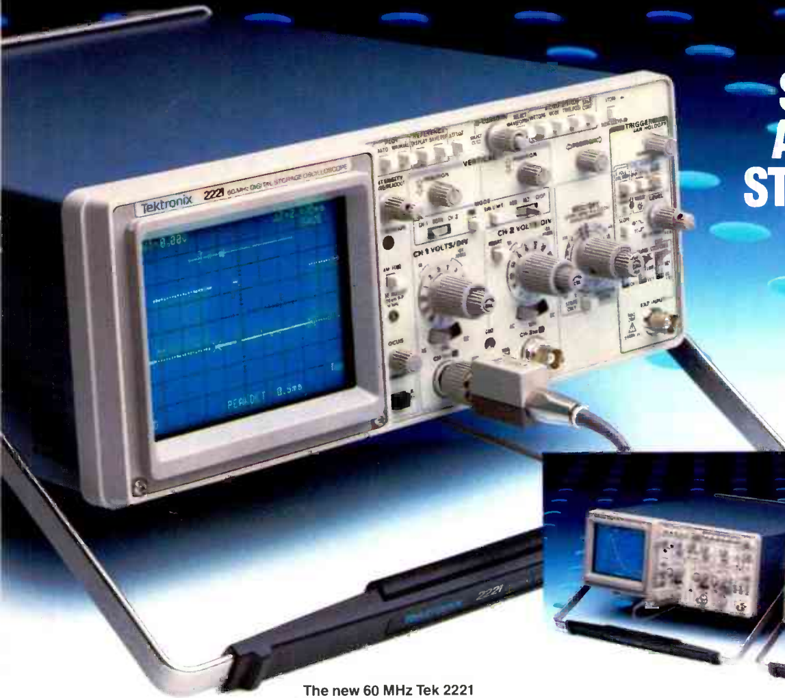
The new 60 MHz Tek 2221 (above) offers such features as CRT readout and measurement cursors for just $3995.
