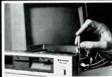
Next, you install the 5¼" floppy disk drive, learning disk drive operation and adjustment. Later, you increase your data storage capacity dramatically by installing a 20 meg hard disk drive.
