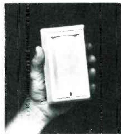
FIG. 6—THIS DUAL-TECHNOLOGY DETECTOR combines passive-infrared and microwave sensors. Other technology combinations can also be used.
